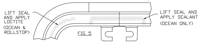
(f) LIFT SEAL AT CORNERS AND APPLY A BEAD OF LOCTITE TO FRAME (fig 5)
