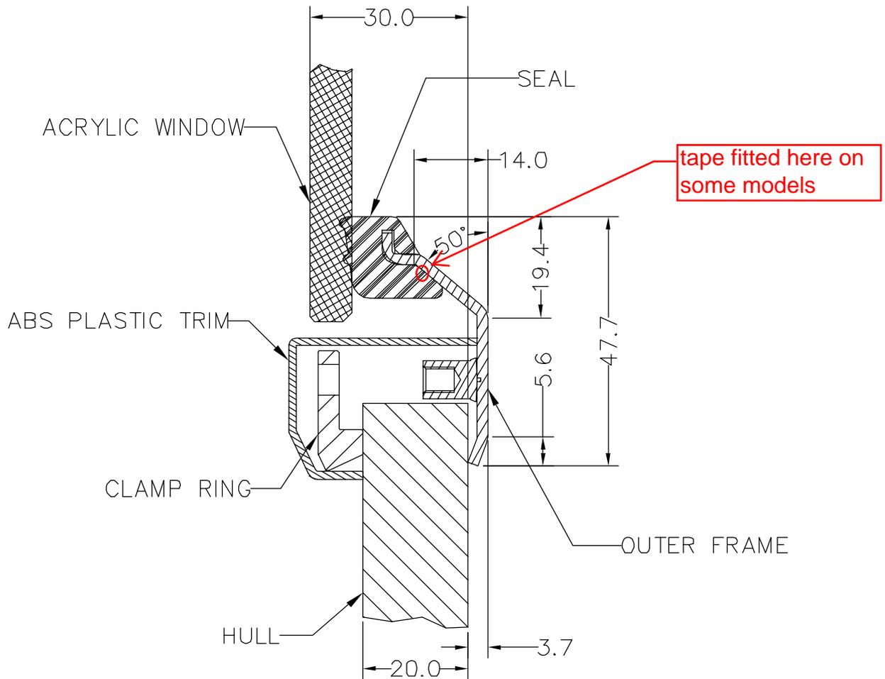
HULL THICKNESS MIN 9mm MAX 30mm
