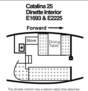
The dinette interior has a saloon table that attaches to the port side of the boat and drops down to form a small berth, and two couches that are on the fore and aft side of the table and face one another across the table.
