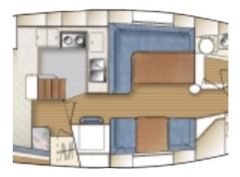
The traditional interior has an "L" shaped seating area on the port side and the table can fold up and store against the forward bulkhead.
