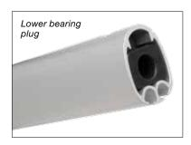
The forestay wire is centred and insulated the full length of the extrusion enabling the extrusion to rotate evenly around the wire. The furling resistance is reduced and chafe between the wire and the extrusion is eliminated.
