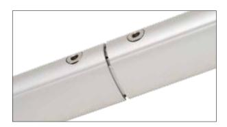
NEW The luff extrusion consists of 2400 mm sections connected with an aluminium joining sleeve and a stainless steel connecting plate. The joining sleeve transmits the torque within the extrusions, and the connecting plates keep the sections together with a slight gap between them. This way chafe is avoided on both the extrusions and the sail.
