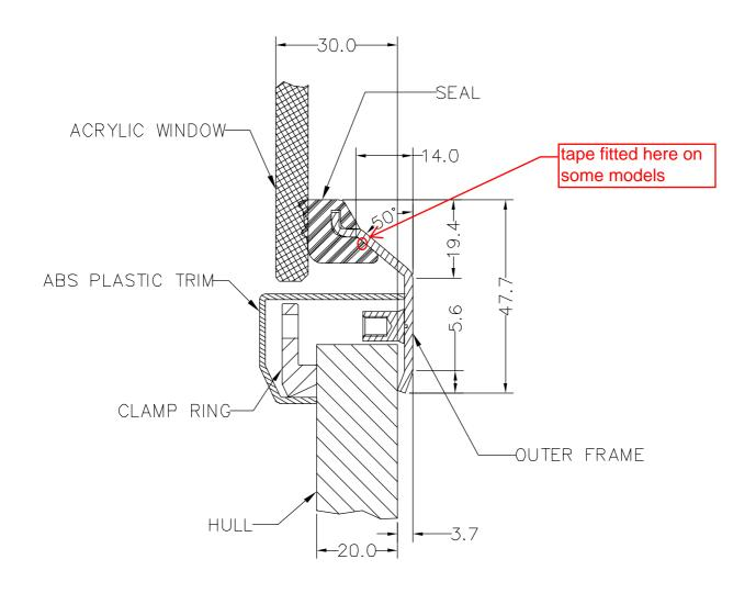
HULL THICKNESS MIN 9mm MAX 30mm FASTENINGS SUPPLIED FOR 17 - 21mm
