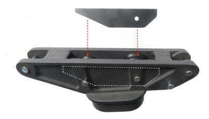
The divider plates have a hole drilled through them that gets mounted between the two forward sheaves in the masthead. The aft end of the divider plate is angled such that it rests on top of the aft pin between the aft sheaves. The divider plate helps prevent the halyards from jumping from one set of sheaves to the other.
