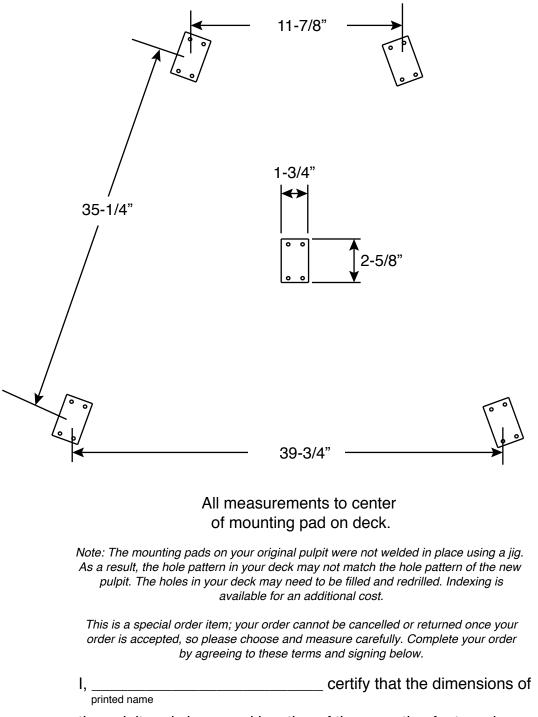
the pulpit and shape and location of the mounting feet as shown in this drawing are correct.
