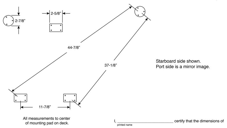
Note: The mounting pads on your original pulpit were not welded in place using a jig. As a result, the hole pattern in your deck may not match the hole pattern of the new pulpit. The holes in your deck may need to be filled and redrilled.
