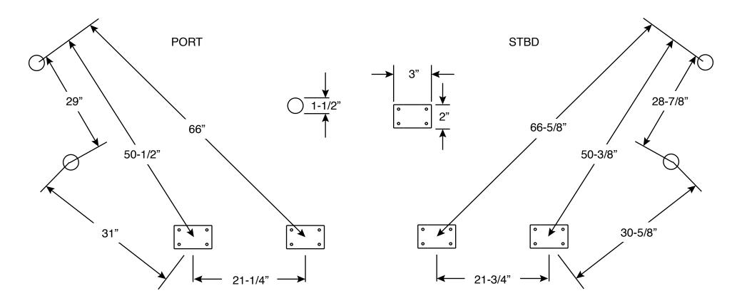
All measurements to center of mounting pad on deck.
