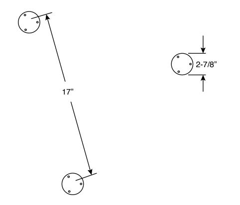
All measurements to center of mounting pad on deck.
