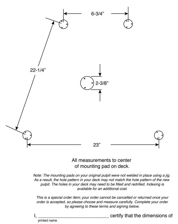
the pulpit and shape and location of the mounting feet as shown in this drawing are correct.
