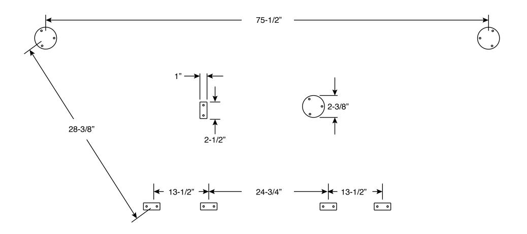
All measurements to center of mounting pad on deck.
