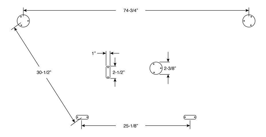
All measurements to center of mounting pad on deck.
