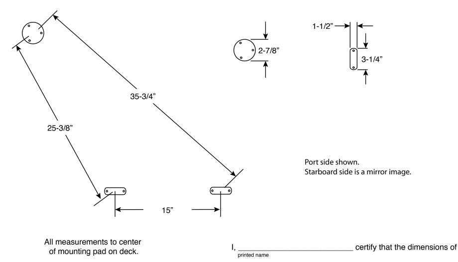
Note: The mounting pads on your original pulpit were not welded in place using a jig. As a result, the hole pattern in your deck may not match the hole pattern of the new pulpit. The holes in your deck may need to be filled and redrilled.
