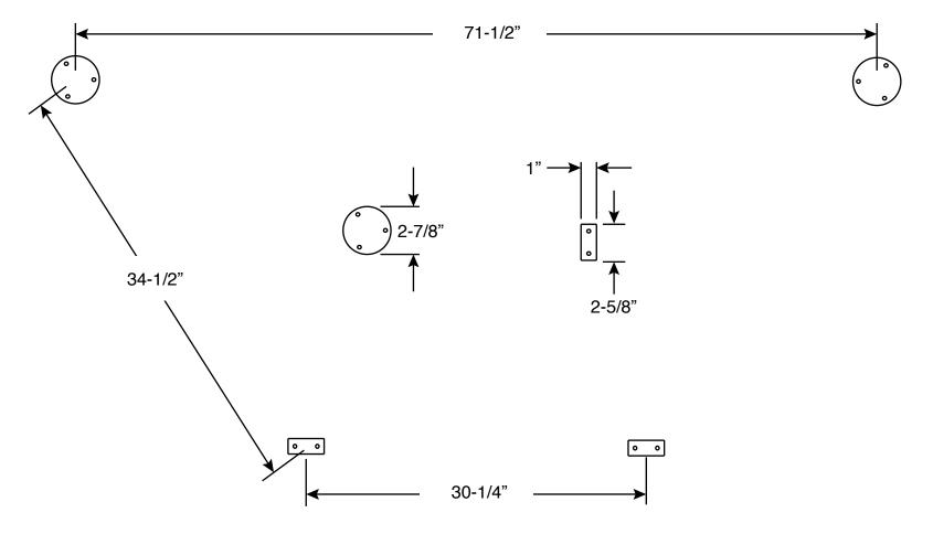
All measurements to center of mounting pad on deck.
