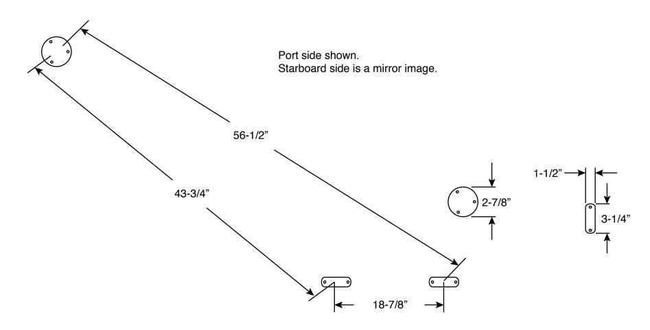
All measurements to center of mounting pad on deck.
