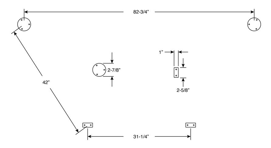
All measurements to center of mounting pad on deck.
