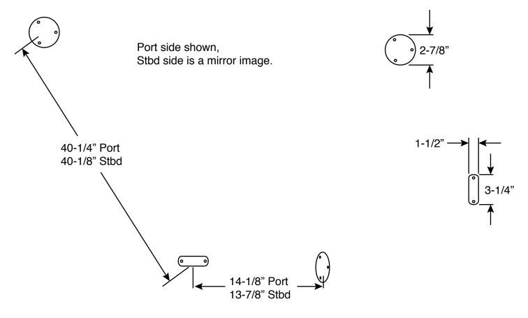
All measurements to center of mounting pad on deck.
