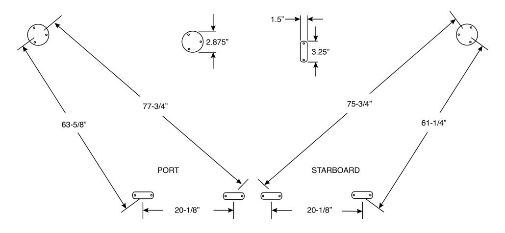
All measurements to center of mounting pad on deck.
