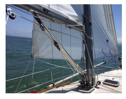
With separate controls, it is typical to have to adjust both the topping lift and boom vang to change the trim of the main or height of the boom. The real beauty of the rigid vang is that a single line does both. You no longer have to ease the vang then haul on the topping lift to raise the boom. Just ease the rigid vang and its spring action raises the boom in one easy motion.
