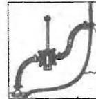
To ensure good priming and flow, avoid sharp bends in pipework and fit a Whale strum-box/strainer (incorporating a non-return valve) which prevents the end of the hose sucking against a flat surface and allows the water level to be reduced to a minimum.
