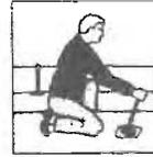
Avoid installations which require a cockpit locker to be opened in order to operate the pump.
